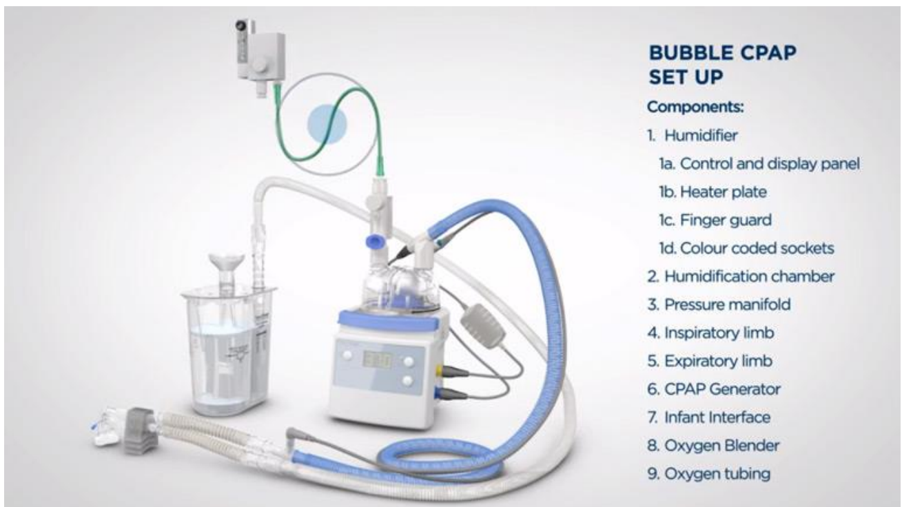
Figure 12.3: Fisher and Paykel Bubble CPAP
